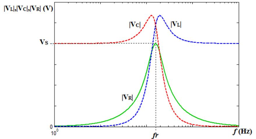
Figure (9)  $|V_c|, |V_L|$  and  $|V_R|$  vs.  $f$
