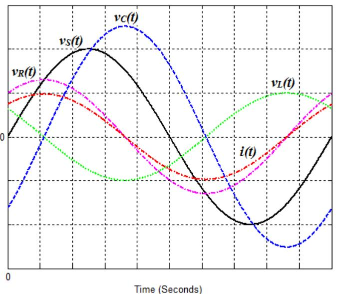
Figure (10) Series RLC Circuit Time Domain Representation
