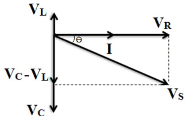
Figure (4) Series RLC Circuit Pharos Diagram when  $f < f_r$
