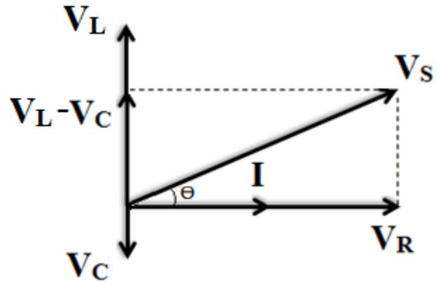
**Figure (5) Series RLC Circuit Phasor Diagram when  $f > fr$**
