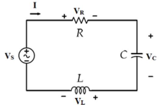
Figure (1) Series RLC circuit
